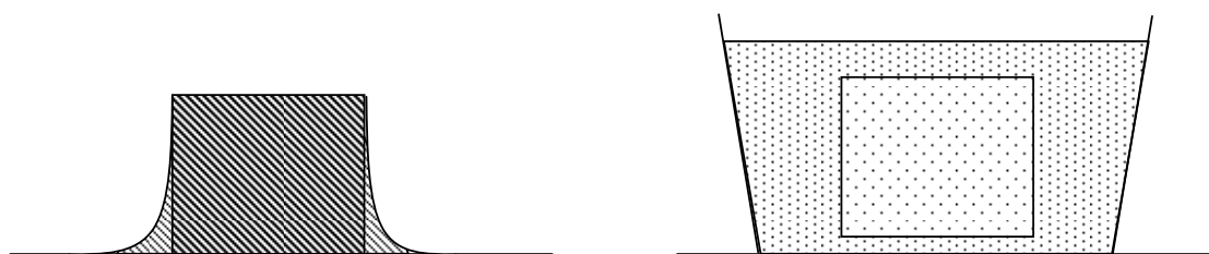
Figure 87. Schematic illustration of the liquor phase and impregnated wood liquor in vapor and liquid phase pulping. The shade of the phases is an indication of the alkali concentration in the different phases during the cooking stage.
